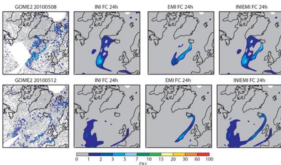
Figure 1 GOME-2 observations (left) and the 24h TCSO<sub>2</sub> forecasts using only initialisation with SO<sub>2</sub> analysis (INI), only the estimates emission parameters (EMI) and a combination of both (INIEMI) for 8 May (top) and 12 May (bottom) 2010 in DU.
